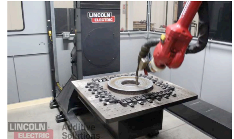
1,600-lb 316-L stainless steel valve body printed using DED-AM (Lincoln Electric)
